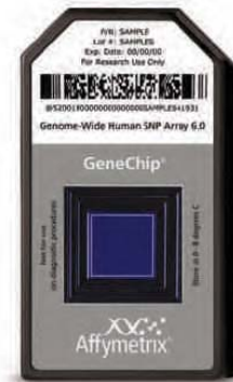
Figure 15.1 Personal genetic testing. Right , a SNP-chip. Personal DNA testing companies use chips like this one to analyze their customers' chromosomes for SNPs. This chip, shown actual size, reveals which versions of 906,600 SNPs occur in the individual's DNA.
