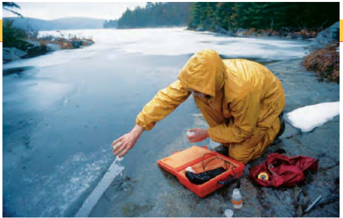
A Biologist testing the pH of water in New York's Woods Lake. In 1979, the lake's pH was 4.8. Since then, experimental addition of calcite to soil around the lake has raised the pH to more than 6.
