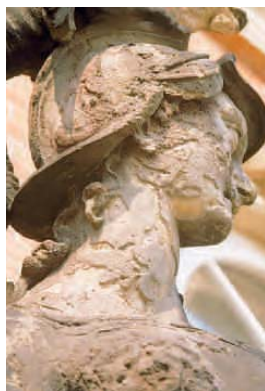
Figure 2.15 Corrosive effect of acid rain. Airborne pollutants dissolve in water vapor and form compounds that change the pH of rain.
